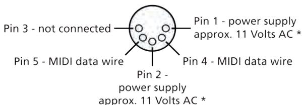
\*: AC voltage is routed to Pin 1 and Pin 2 only when the Phantom Power switch is engaged.
