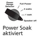
**26 Power Range Selector:** Use this switch to activate the *Power Soak* and select the desired power level. The *Power Soak* works only in combination with the amp's 8-Ohm Output (23)! You have four options:
