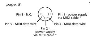
\*: Power supply from ENGL devices that are equipped with a MIDI IN port. The corresponding configuration switch at the amp must be set to the position ENGL MIDI Footcontroller.
