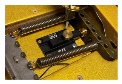
6. After tightening the remaining screws, reinsert the spring.
